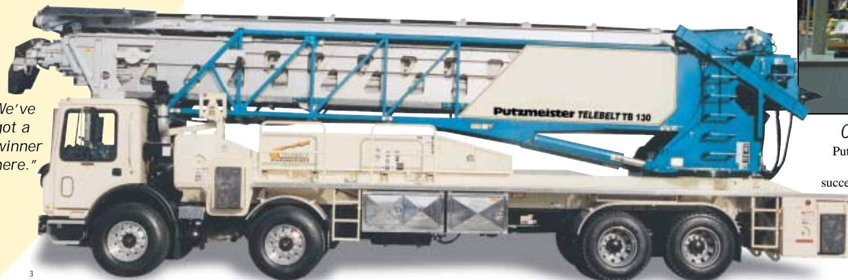
Kiewit uses the TB 130 on a powerhouse pour in Grand-Mere, Quebec on December 6, 2001. The unit placed 425 cubic yards of 2.5" aggregate at a 2" to 3" slump concrete.
