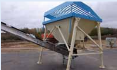
The attached grate prevents the introduction of foreign material into the hopper.
