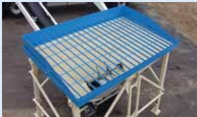
A hydraulically-controlled auger keeps flowable fill entering the hopper moving smoothly onto the feeder belt.
