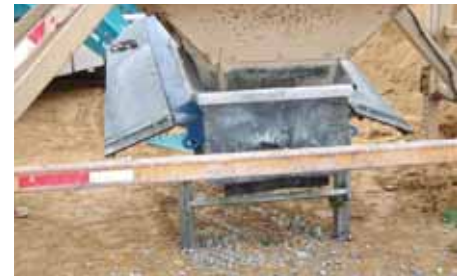
The Rock Hopper/Low Profile Hopper combination keeps the tail pulley off the ground. The reduced feeder angle offers greater efficiency.
