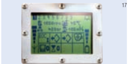
The clear display on the remote control provides up-to-date feedback and system information about the machine. Various parameters can be set here. The strength of the radio signal and charge status of the battery is indicated via bars.
