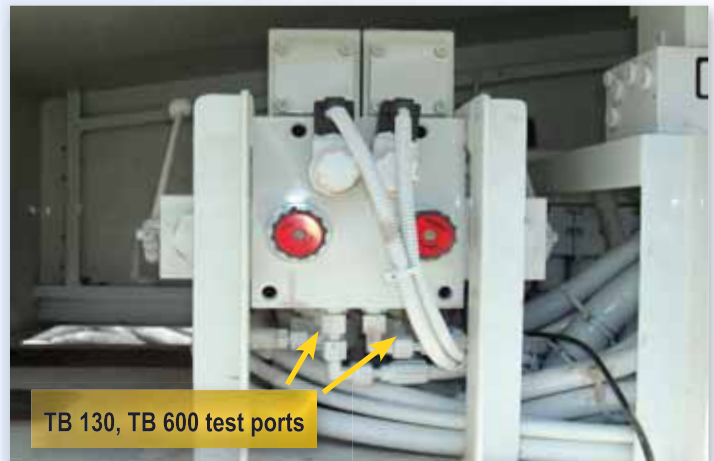
Figure 2 Above shows the TB 130 and TB 600 controls. Controls on the TB 130 and TB 600 are “laid down” so the volume control knobs face you. As a result, the TB 130 and TB 600 port M1A and port M2A face downward.
